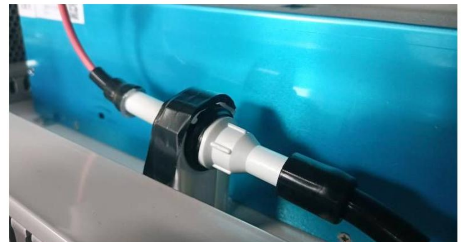
Insulation Support Frame
