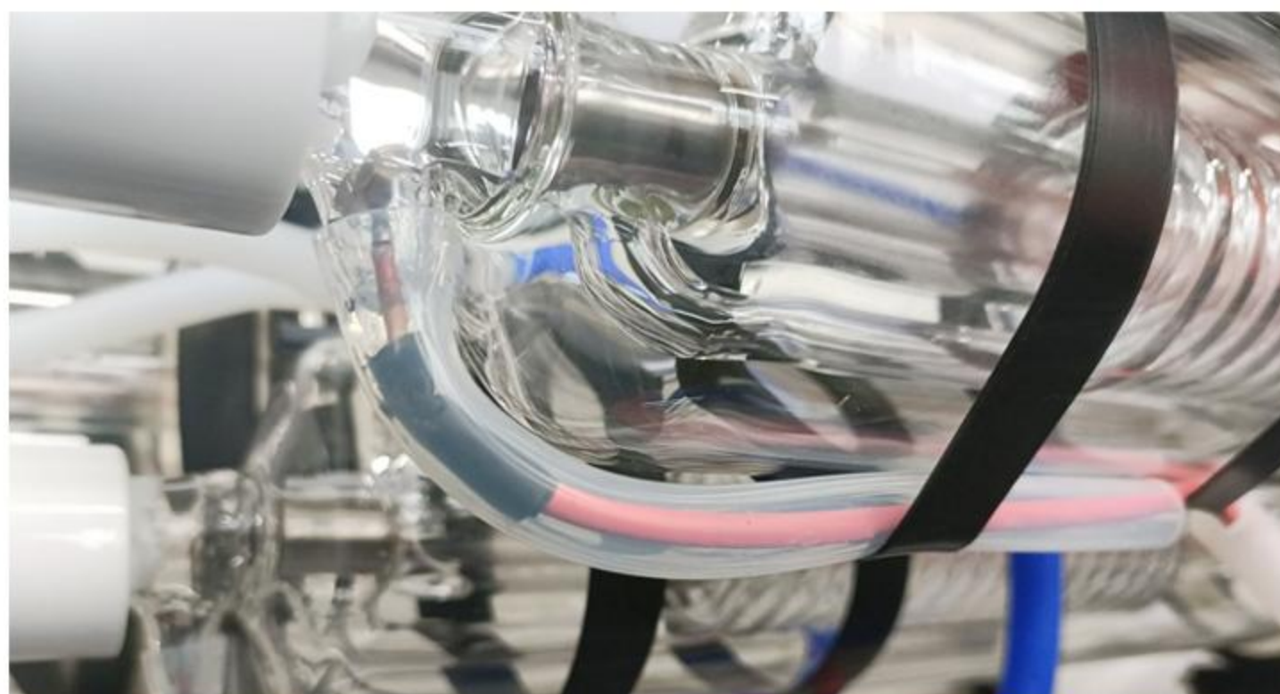
High-Voltage Wire Insulation
