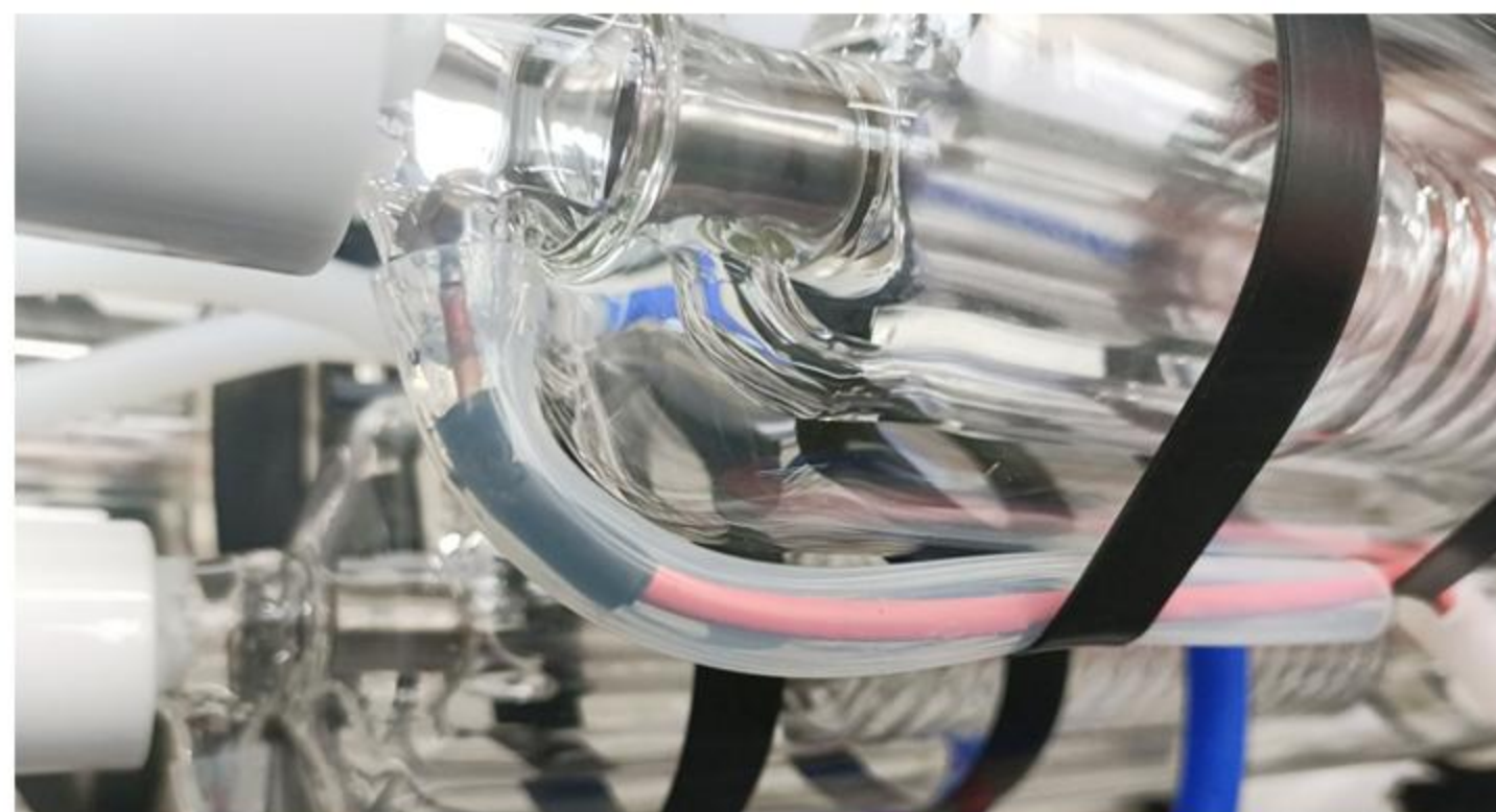
High-Voltage Wire Insulation
