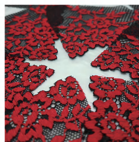
Hot sealed edge cutting
