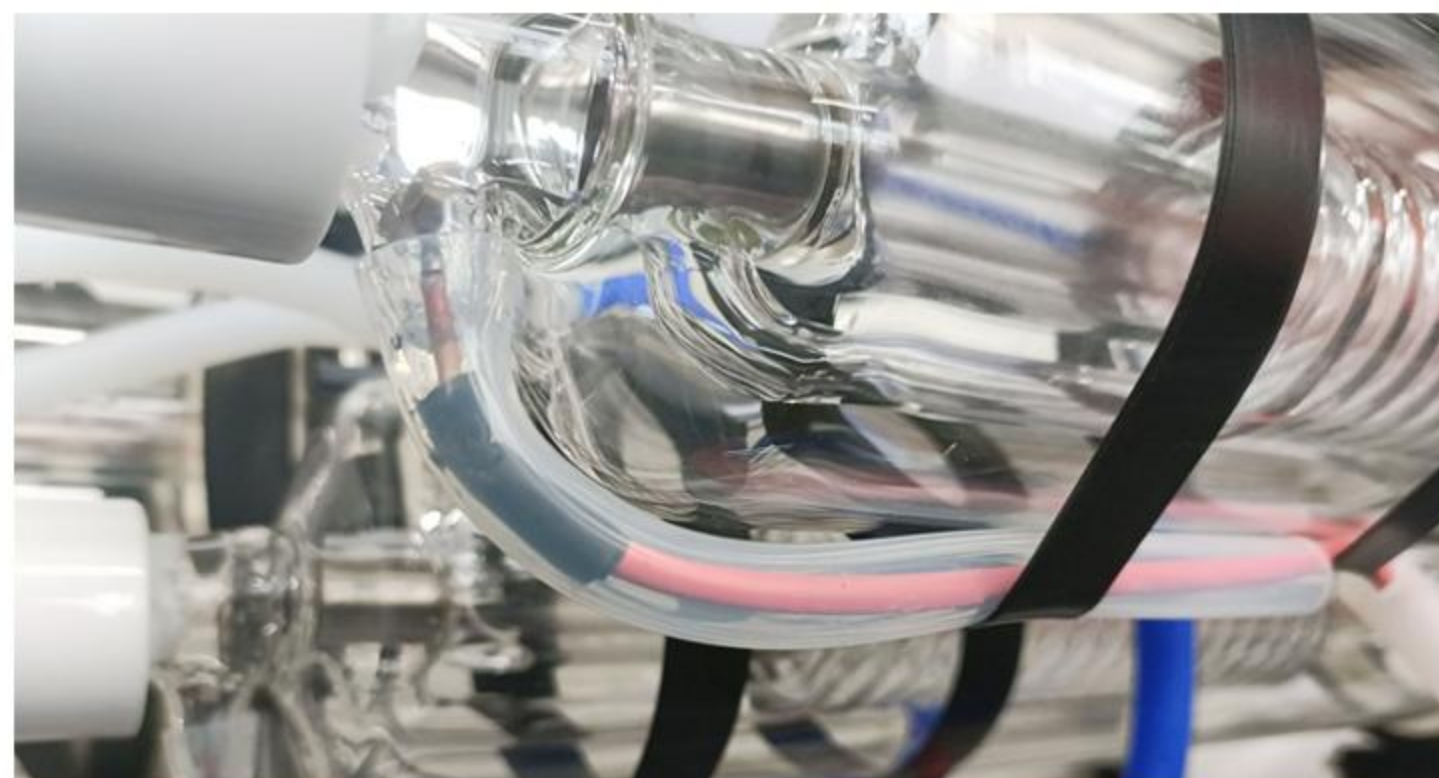
High-Voltage Wire Insulation
